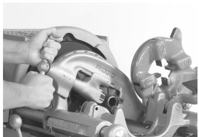
Figure 5 – Cutting Pipe with 820 Cutter
