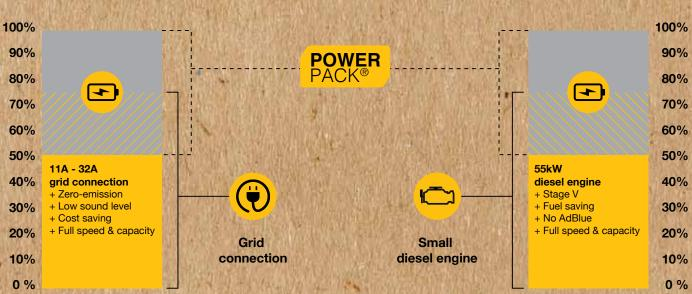
To operate the crane in electric mode it needs to be connected to a grid connection which is often available at most job sites. The system can be operated between 11A and 32A which can be pre-set at the display, so there still can be energy left for other equipment on site. The surplus energy of the grid connection is used to recharge the battery of the PowerPack®, so it can be used for peak absorption.
