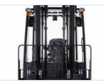
The neatly arranged hydraulic hoses and chains provide clear front visibility through the wide view mast.
