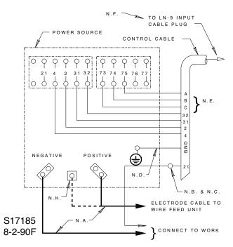
Above diagram shows electrode connected positive. To change polarity, turn power off, reverse the electrode and work leads at the power source, position the positive-negative switch on the power source to correspond to the polarity of the electrode cable connection. Refer to LN-9 operating manual for required polarity connections.
