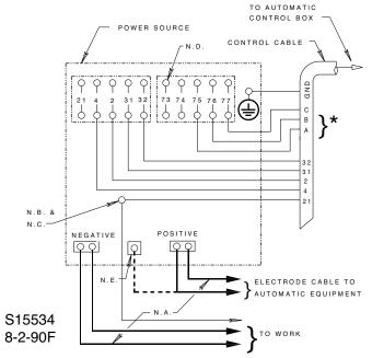
Above diagram shows electrode connected positive. To change polarity, turn power source off, reverse the electrode and work leads at the power source and position the switch on power source to proper polarity. Also reverse the leads on the back of the ammeter and voltmeter in the automatic control box. Connect the control cable ground lead to the frame terminal marked near the power source terminal strip. The power source must be properly grounded.
