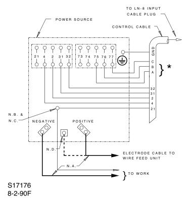
Connect the control cable ground lead to the frame terminal marked hear the power source terminal strip. The power source must be properly grounded.
