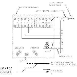
Above diagram shows electrode connected positive. To change polarity, turn power off, reverse the electrode and work leads at the power source and position the switch on power source to proper polarity.
