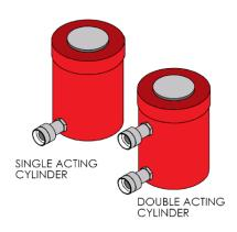
Connect the hoses between the cylinder and the pump ensuring that the coupling/s are fully **hand tightened** only. **Never** use wrenches to attempt to connect the coupling/s, incorrectly connected coupling/s is one of the most common causes of faulty operation.
