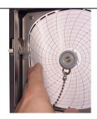
Make sure that the chart is placed under the chart clips 4x for case 192x192 mm 3 x for case 280x280 mm 4 x for case 380x380 mm 4 x for case 463x335 mm on the lower panel.
