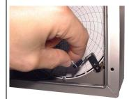
Remove the protective cover of the recorder pen.
