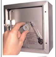
Open the recorder door and remove the knob of the clockwork by turning it clockwise.
