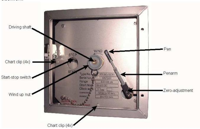
Above is shown the important parts required to operate the recorder properly. A extra dial with pointer is available as an option. Also other colour fibre pens can be ordered.
