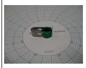
Return the knob of the clockwork by turning it anticlockwise. Wind up max. 5 turns!
